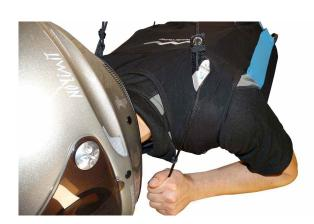
The dual suspension strap is moved towards the pelvis with 2 straps when the harness is tensioned with the legs, and stays in that position throughout the flight.
