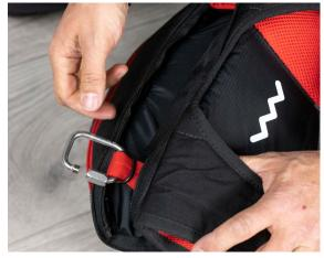
The two connections must be made with screw carabiners with a breaking load of at least 1400 Kg. In any case, it must be verified that the length of the bridle line is sufficient to position the reserve parachute inside the harness's built-in container and that there remains enough slack to allow for the extraction of the reserve parachute without causing the deployment of the launch bag during extraction.
