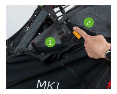
In detail, adjustment n°1 varies the angle between the legs and the back (seat depth), distributing the loads between the seat and the lumbar strap, thus providing greater comfort to the pilot. The main adjustment that allows you to choose the inclination of the torso in relation to the vertical axis of flight is n°2, for back adjustment.
