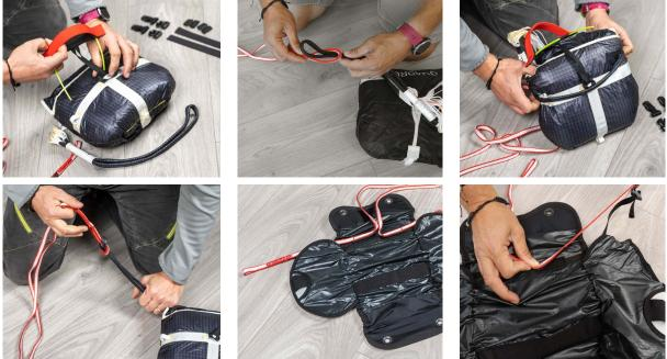
The bridle of the container has a Velcro designed to be fastened with the container. Once the bridle is connected, insert the parachute and its bundle into the container while keeping the handle facing upward To close the flaps of the container, you can use a thin cord (such as a paragliding line) and insert it through each elastic loop. With the help of this cord, you will be able to close the container securely.
