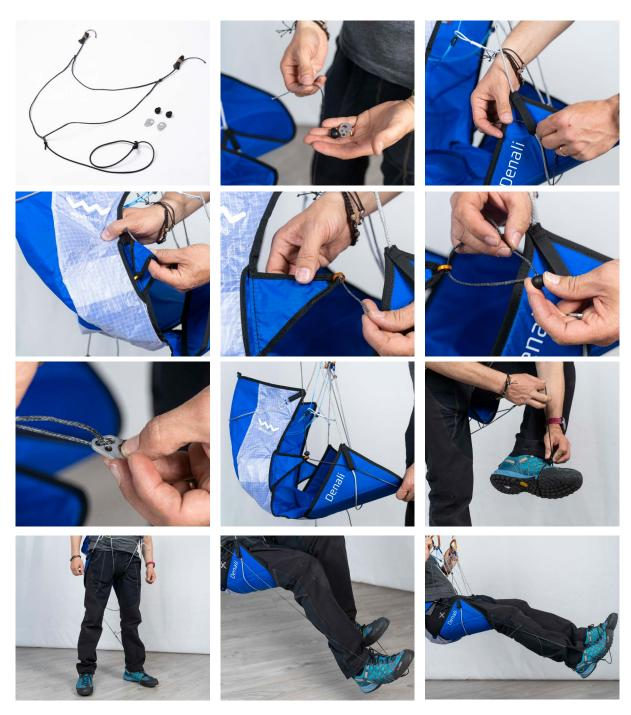
If the accelerator is not used, it is advisable to close the side flaps with the ring in the appropriate pockets.
