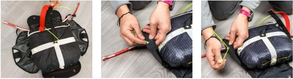
Insert the elastic loops through the eyelets of the upper flap and then into the lower one, proceed by fixing the pins of the handle in the respective elastic loops at the end remove the thin cord. Secure the handle to the container with the velcro, so that it maintains the ideal position and avoids accidental opening, and lastly insert the two pins into the holes in the lower flap.
