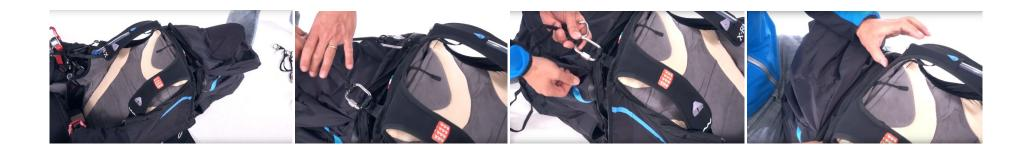
The two connections should be made using screw-lock karabiners with a breaking strength of at least 1,400 kg. It is important to verify that the length of the bridle is sufficient to position the reserve parachute inside the harness pocket, and that there is sufficient play to enable the parachute to be taken out of the pocket without causing the reserve parachute deployment bag to open during extraction.
