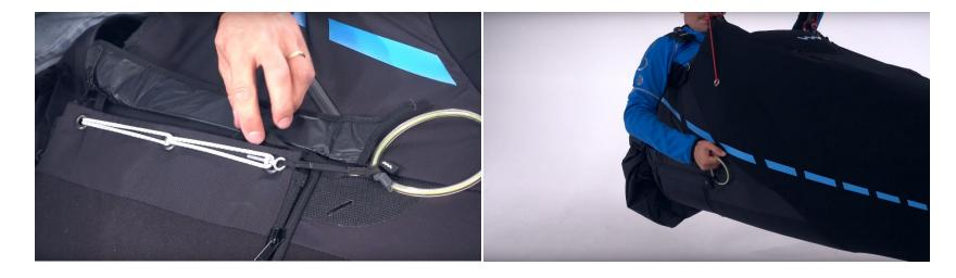
It is essential to remove the cords after this operation. The cords should be pulled out slowly in order not to damage the elastic loops by excessive friction.
