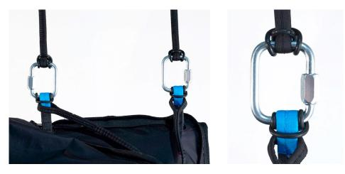
The two connections should be made using screw-lock karabiners with a breaking strength of at least 1,400 kg. It is important to verify that the length of the bridle is sufficient to position the reserve parachute inside the harness pocket, and that there is sufficient play to enable the parachute to be taken out of the pocket without causing the reserve parachute deployment bag itself to open during extraction.
