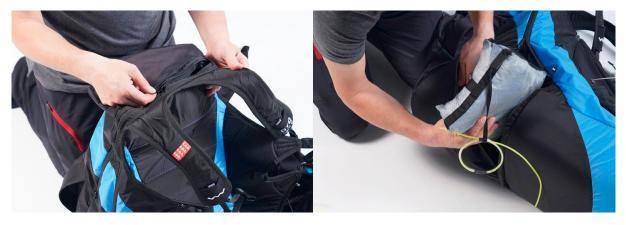
Insert the elastic loops in the corresponding pockets and through the small eyelets. Insert the parachute in the harness container with rescue handle facing upwards and rescue parachute lines facing the harness tail.
