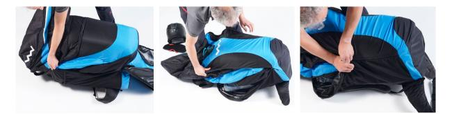
Once the harness is inserted, turn over the entire package and close the zipper. Fold the tail inside. The materials used allow any extent of folding without affecting how it functions in flight. Enough space will be available in the top part for the instruments and helmet.
