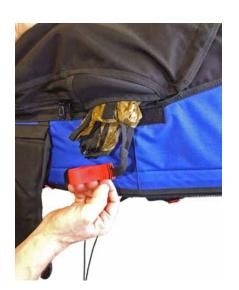
This system will allow you to deploy your braking parachute holding it firmly in your hand while approaching landing and then to release it precisely at the most opportune moment. If you want immediate opening simply release the handle immediately after deployment.
