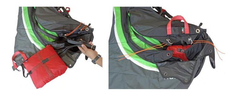
Adjust container volume according to the dimensions of the parachute, using the eyelets at the ends of the elastic fabric. If the parachute is small in size, use the eyelet closest to the parachute itself while, if the parachute is large, use the other eyelet. To close the two elastic fabric flaps, cross them over so as to maintain the parachute as close as possible to the seat.
