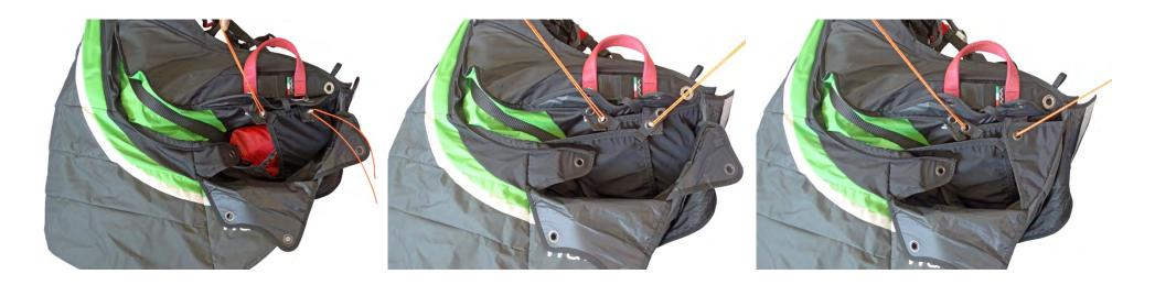
Take the bridle cover zip all the way to the right to close it, moving the zip about 20 cm leftward. Then begin to close the outside parts of the container, following the progressive order in the photographs, taking care during this phase that the zip does not open back up at the right end. Introduce the handle's metallic pins into the elastic loops and under the transparent cover.
