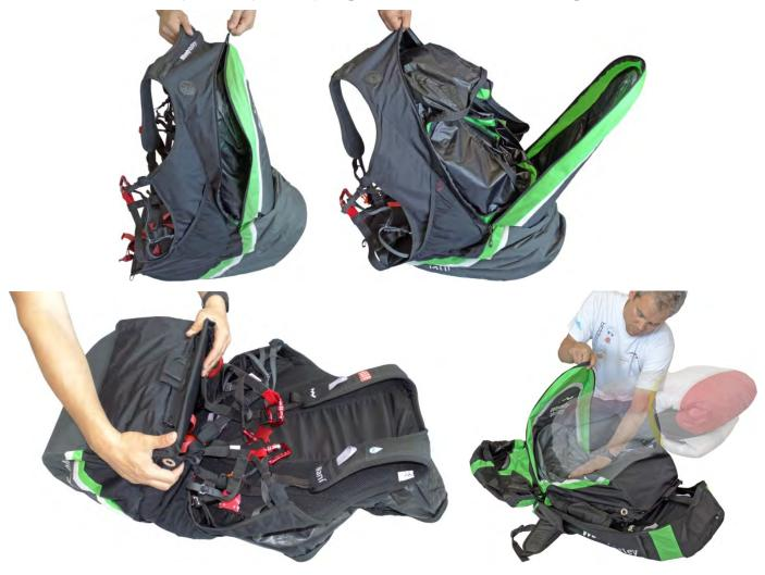
Place the paraglider above the rear pocket and, finally, close the backpack. For easier zipper closing, crush the backpack so as to remove remaining air inside the paraglider and the airbag.
