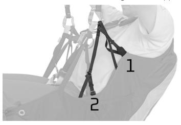
If you want to change the adjustments you must first alter adjustment No. 1 to the most comfortable point. Once this step is completed, adjust the No. 2 seating depth belt to reach the new position desired.
