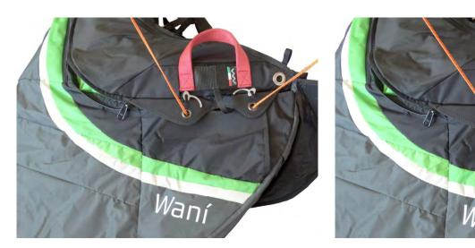
After having closed all container parts, it is advisable to check that the zip part under the opening system has been closed correctly.
