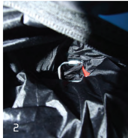
(1) "Anti-G" side pocket, (2) karabiner for attaching the drag chute bridle (3-4). Example of extracting the parachute (5-6).
