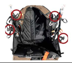
When connecting the reserve parachute to the harness, ensure that the parachute bridle passes outside the harness' main attachment strap and then to the karabiner.
