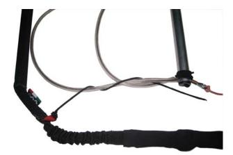
Lastly, tie the elastic cord to the loops on the speed system. This procedure ensures that the SPEED-SYSTEM is taut, ready for use, and above all neat and tidy.
