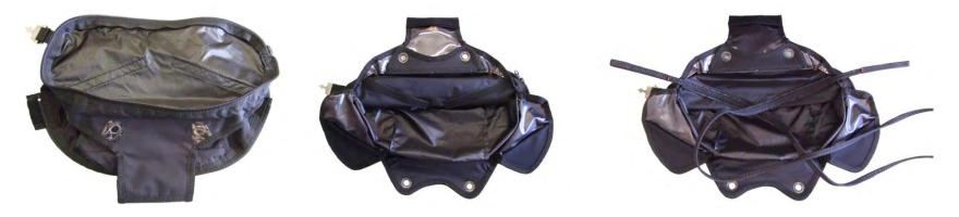
Insert the parachute into the harness container so that the deployment handle is visible and facing outwards, and with the loop that connects the handle to the deployment back facing upwards. Thread a thin cord (such as a paraglider shroud line) into each elastic loop. This will make it easier to close the container.
