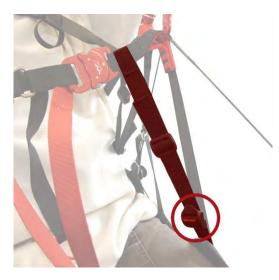
This adjustment affect flying performance. The looser it is, the less stable the harness becomes, and therefore the more sensitive to pilot movements. Vice versa, the tighter it is adjusted, the more stable the harness becomes, requiring more pronounced pilot movements in flight.
