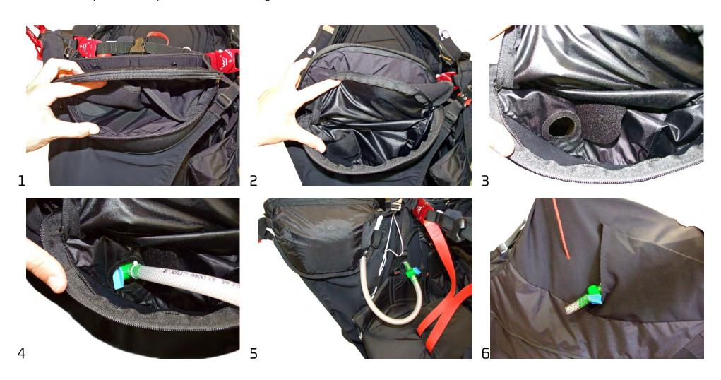
Open the zipper beneath the instrument compartment (1) to access the ballast lodging (2). Next, open the Velcro over the discharge tube's outlet hole (3) and insert the tube (4). There is a second through-hole (5) inside the harness, which allows the discharge tube to be inserted into the external pocket, where it can be hidden and extracted whenever necessary (6).
