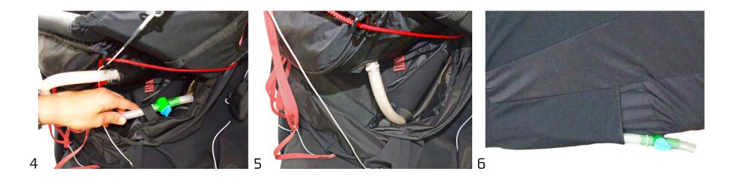
Insert the tube into the slot on the right hand side (4) and slide it through the hole that leads from the inside of the harness (5) to the pocket on the outside, from which the tap can be extracted for drainage (6).
