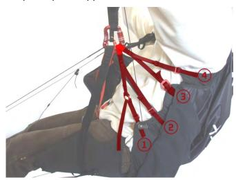
In the detail photo, adjustment n° 1 changes the angle between thighs and back (seat depth), distributing load between seat and the lumbar area and thus improving pilot comfort.
